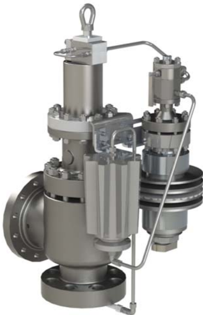
Series 9000/604 Pilot operated safety valves for superheated water and steam. Flanged inlet and outlet connections. Orifices: D to T 2 Materials: carbon or alloy steel Set pressure range: 10 to 300 bar Temperature limit: 375 °C Overpressure: 3% Blowdown: 4%
