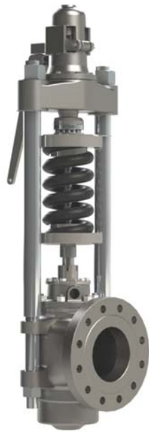
Series 200 High pressure steam safety valves with inlet prepared for welding or flanged. Orifices: G to R 4 Materials: carbon or alloy steel Set pressure limit: 360 bar Temperature limit: 649°C Overpressure: 3% Blowdown: 4%
