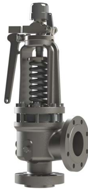
Series 300S Low and medium pressure steam safety valves. Flanged inlet and outlet connections. Orifices: H to R 1 Materials: carbon or alloy steel Set pressure range: 1.5 to 80 bar Temperature limit: 543°C Overpressure: 3% Blowdown: 4%
