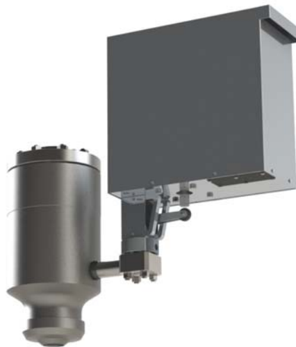
Series 100 - TAIMATIC Electrically operated safety valves for steam service. Sizes: 2.5" x 4" Material: alloy steel Set pressure limit: 310 bar Temperature limit: 621°C Overpressure: none Accuracy of opening pressure: ± 1% Supply voltage: 110/125/220 Vdc, Vac and other voltages available
