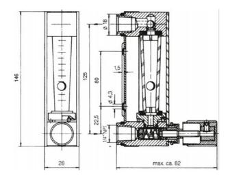
The upper edge of the float is the reading edge.
