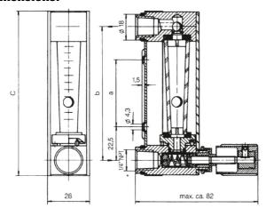
The upper edge of the float is the reading edge.
